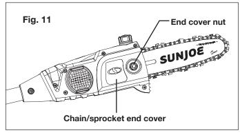
**NOTE:** If the chain is too tight, it will not rotate. Loosen the end cover nut slightly and turn the chain tensioner 1/4 turn counterclockwise. Lift the tip of the guide bar up and retighten the end cover nut. Ensure that the chain can be rotated by hand without binding.
