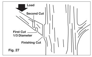
Now make your finishing cut from the topside of the branch smoothly and neatly against the main member so the bark will grow back to seal the wound.  Release the trigger ON/OFF switch as soon as the cut is completed. Failure to follow proper cutting procedures will result in the bar and chain binding and becoming pinched or trapped in the limb.
