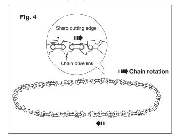
**5.** Starting at the tip, mount the chain drive links into the bar groove, leaving a loop at the back of the bar. The chain will loosely fit until it is placed on the sprocket. (Figs. 5 & 6)
