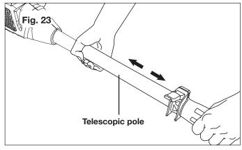
4. Lock the pole in position by closing the cam-lock (Fig. 24), and ensure that the pole is secure. If the pole telescopes when the cam-lock is closed, the nut may need tightening.
