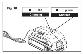
**NOTE:** If the charger plug light remains green while the charger base light alternately flashes red and green, this indicates a temperature abnormality (i.e. that the battery pack is either too hot or too cold).
