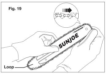
6. Mount the guide bar by inserting the studs into the long slot on the guide bar; arrange the chain loop on the back of the bar to ensure the sprocket is inserted in the loop (Fig. 20).
