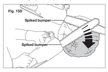
When bucking on a slope, always stand on the uphill side of the log. When cutting through the log, maintain control by releasing the cutting pressure near the end of the cut without relaxing your grip on the chain saw handles. Do not let the chain contact the ground.
