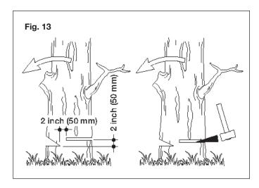
Make the lower horizontal notching cut first. This will help to avoid pinching either the saw chain or the guide bar when the second notch is made.
