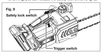
5. To turn the tool off, simply release the trigger switch.
