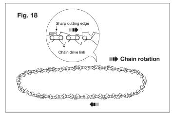
5. Starting at the tip, mount the chain drive links into the bar groove, leaving a loop at the back of the bar. The chain will loosely fit until it is placed on the sprocket (Fig. 19).
