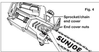
2. Lift up the guide bar tip slightly. Use the other end of the hex key wrench/blade screwdriver to turn the chain adjusting screw clockwise to tighten, turn it counterclockwise to loosen. A cold chain will be correctly tensioned when there is no slack on the underside of the guide bar; the chain is snug, but it can be turned by hand without binding (Fig. 5).
