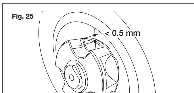
Do not mount a new chain with a worn sprocket or vice-versa.
