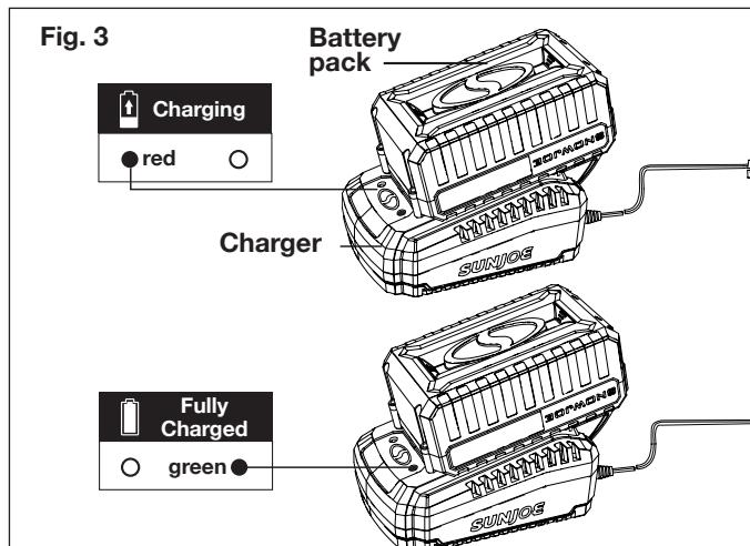
4. When the charger light turns green, the battery is fully charged (Fig. 3).
