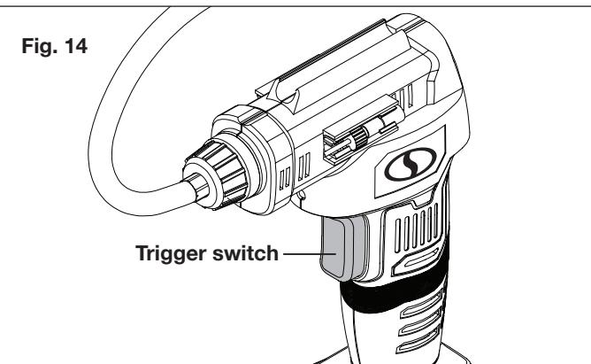
6. To turn the compressor OFF, press the trigger switch (Fig. 14).
