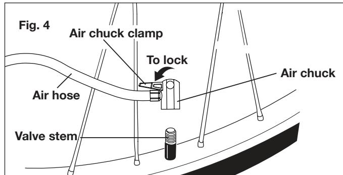
4. To remove, lift air chuck clamp and remove air chuck from valve stem (Fig. 5).
