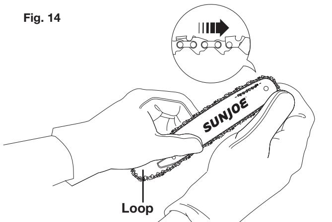
6. Hold the chain in position on the bar and place the loop around the sprocket. Fit the bar against the mounting surface so that the extruded piece on the mounting surface is in the long slot of the bar and the adjusting pin is in the chain tension pin hole (Fig. 15).
