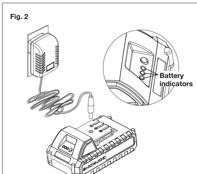
3. The battery will take approximately 5 hours to charge. The battery indicator LEDs will twinkle and illuminate one by one during the charging process. Unplug the charger immediately when the 3 LEDs are all illuminated.
