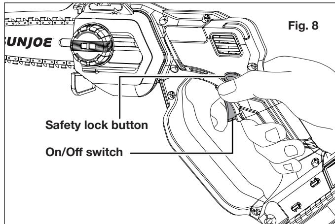
4. To turn the tool off, simply release the On/Off switch.
