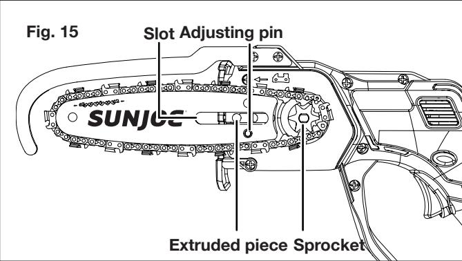
7. While keeping the bar and chain against the mounting surface, adjust the chain tension as needed by adjusting the chain tensioner screw with the supplied hex key wrench. Turn the chain tensioner screw clockwise to tightening the chain, or counter-clockwise to loosen the chain (Fig. 4).
