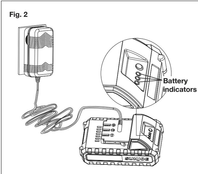
3. The battery will take approximately 80 minutes to charge. The battery indicator LEDs will twinkle and illuminate one by one during the charging process. Unplug the charger immediately when the 3 LEDs are all illuminated.
