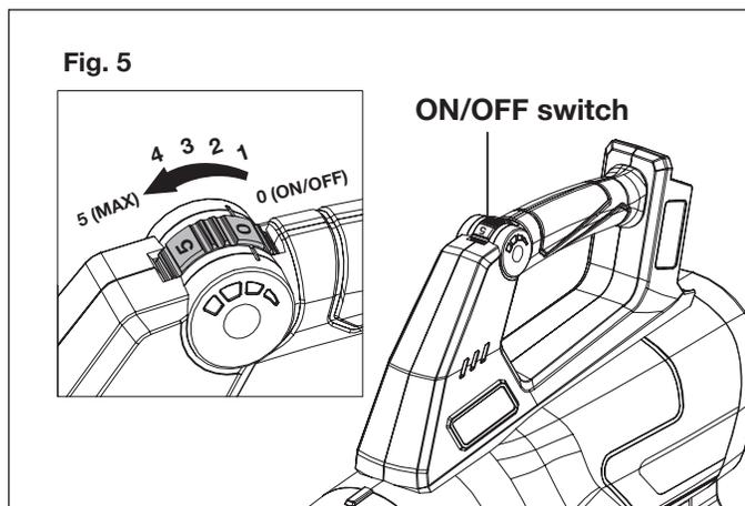
3. This unit is equipped with 5 variable speed settings. Position "5" is the maximum setting blow up to 100 mph (Fig. 6).
