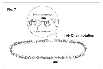
Starting at the tip, mount the chain drive links into the bar groove, leaving a loop at the back of the bar. The chain will loosely fit until it is placed on the sprocket (Figs. 8 – 9).
