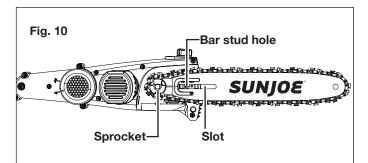
7. Replace the chain/sprocket end cover by positioning the cover onto the saw head. Fit the end cover knob by inserting the bar stud into the bar stud hole. Tighten the end cover knob, but leave the bar free to move for tension adjustment (Fig. 11).
