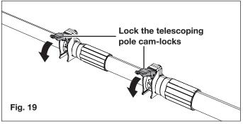
**WARNING!** Failure to lock the telescoping pole camlocks as directed could result in personal injury.
