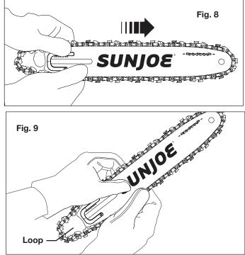
**6.** Hold the chain in position on the bar and place the loop around the sprocket. Fit the bar flush against the mounting surface so that the bar stud hole are aligned with the long slot of the bar (Fig. 10).
