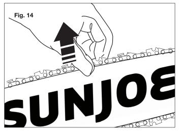
**NOTE:** If the chain is too tight, it will not rotate. Loosen the end cover knob slightly and turn the chain tension knob 1/4 turn counterclockwise. Lift the tip of the guide bar up and retighten the cover cap knob. Ensure that the chain can be rotated by hand without binding.
