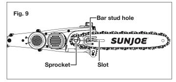
7. Replace the chain/sprocket end cover by positioning the cover onto the saw head. Fit the end cover knob by inserting the bar stud into the bar stud hole. Tighten the end cover knob, but leave the bar free to move for tension adjustment (Fig. 10).
