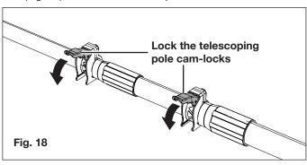
**WARNING!** Failure to lock the telescoping pole camlocks as directed could result in personal injury.
