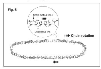
5. Starting at the tip, mount the chain drive links into the bar groove, leaving a loop at the back of the bar. The chain will loosely fit until it is placed on the sprocket (Figs. 7 – 8).
