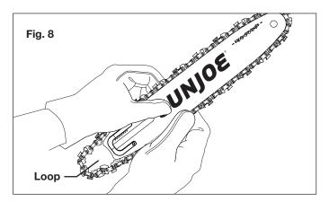
6. Hold the chain in position on the bar and place the loop around the sprocket. Fit the bar flush against the mounting surface so that the bar stud hole are aligned with the long slot of the bar (Fig. 9).
