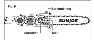
7. Replace the chain/sprocket end cover by positioning the cover onto the saw head. Fit the end cover knob by inserting the bar stud into the bar stud hole. Tighten the end cover knob, but leave the bar free to move for tension adjustment (Fig. 10).
