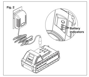
**3.** The battery will take approximately 5 hours to charge. The battery indicator LEDs will twinkle and illuminate one by one during the charging process. Unplug the charger immediately when the 3 LEDs are all illuminated.
