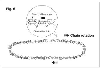
Starting at the tip, mount the chain drive links into the bar groove, leaving a loop at the back of the bar. The chain will loosely fit until it is placed on the sprocket (Figs. 7 – 8).
