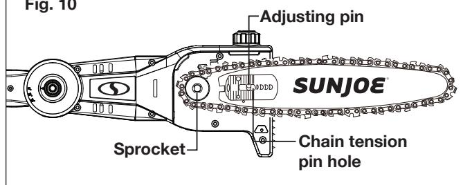
8. Replace the chain/sprocket end cover by positioning the cover onto the saw head. Tighten the end cover knob, but leave the bar free to move for tension adjustment. Put back the hex bolt by screwing it clockwise with the hex key wrench.
