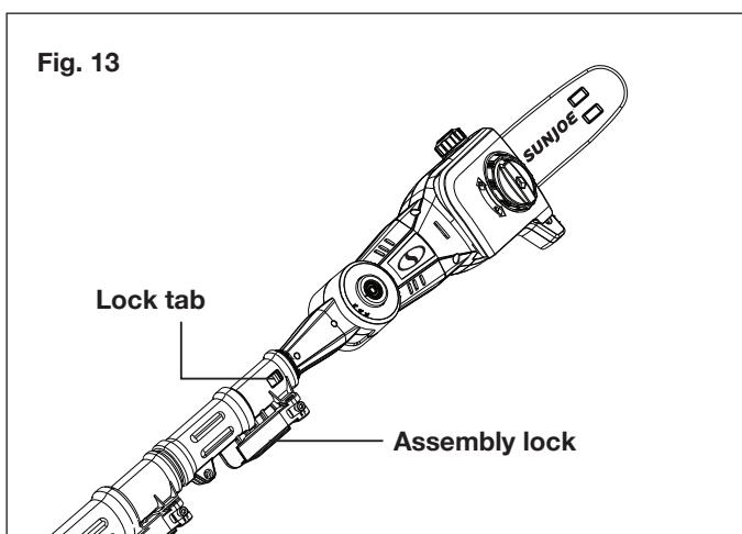
3. To remove the chain saw head, release the On/Off trigger switch and remove the battery. Unlock the assembly lock. Push the lock tabs on both sides, and pull the chain saw head out (Fig. 13).
