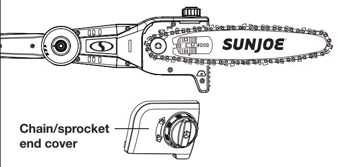
3. Remove the bar and chain from the mounting surface (Fig. 6).
