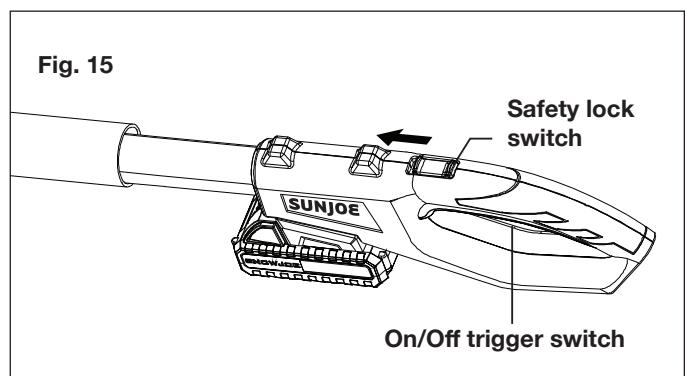
3. To turn the tool OFF, release the On/Off trigger switch (Fig. 15).
