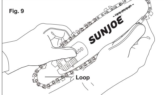
7. Hold the chain in position on the bar and place the loop around the sprocket. Fit the bar flush against the mounting surface so that the bar studs are in the long slot of the bar and the adjusting pin is in the chain tension pin hole (Fig. 10).
