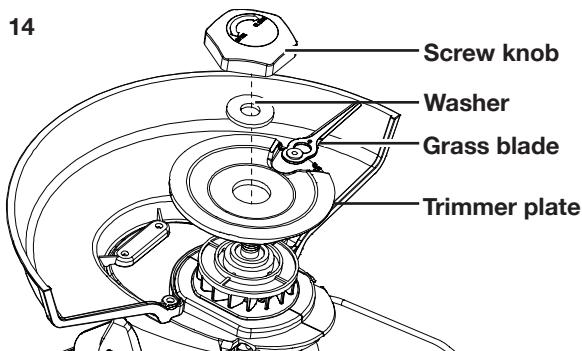
4. Assemble the new SharperBlade™ to the cordless grass trimmer + edger with the washer placed in the middle (Fig. 14). Fix the whole assembly with the screw knob. Twist clockwise to secure.
