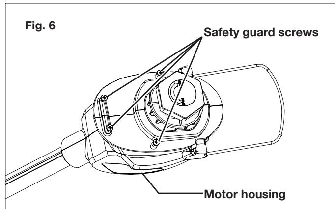
2. Place the safety guard over the motor housing as shown. Align the holes. Fix with the original 4 safety guard screws. Tighten to secure (Fig. 7).
