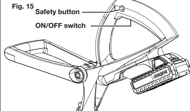
2. To switch OFF, release the ON/OFF switch (Fig. 15). Remove the battery.
