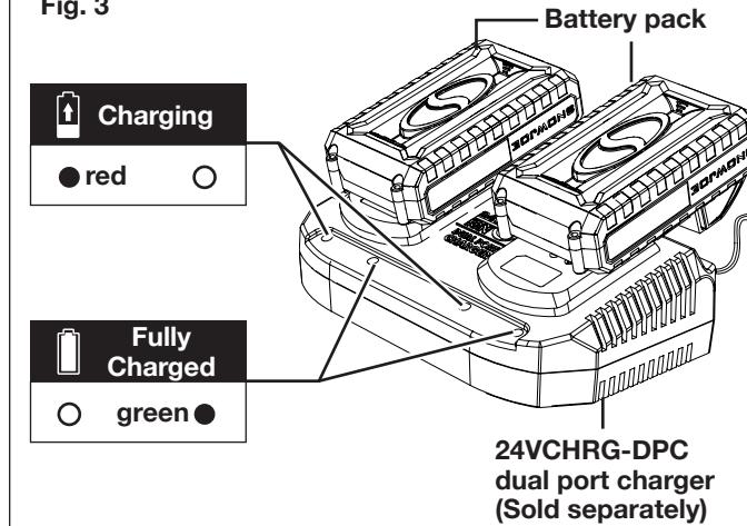
3. The battery indicator LEDs will illuminate one by one during the charging process. Unplug the charger immediately when the 3 LEDs are all illuminated.
