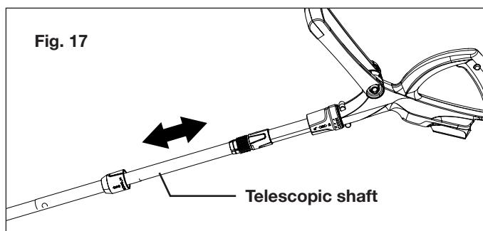
4. Tighten the knob to lock the pole (Fig. 16).
