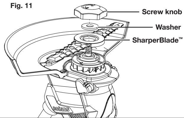
3. Assemble the new SharperBlade™ to the cordless grass trimmer + edger with the washer placed in the middle (Fig. 11). Fix the whole assembly with the screw knob. Twist clockwise to secure.
