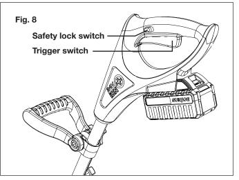
**3.** To stop the cordless snow shovel, release the trigger switch.
