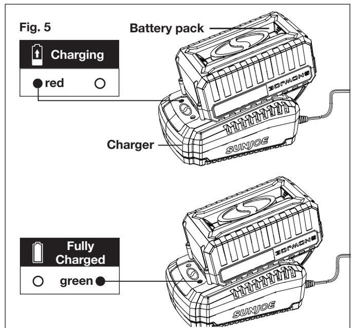
4. When the charger light turns green, the battery is fully charged (Fig. 5).
