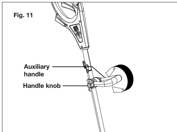
3. Fix the handle by tightening the handle knob. Insert the battery and resume working.
