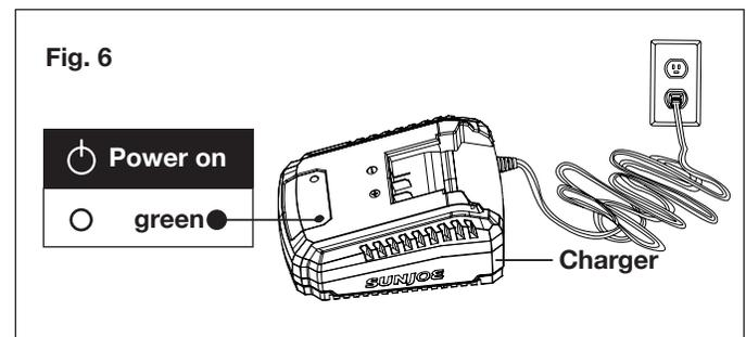
3. Place the battery pack into the charger by sliding the pack to lock it into position. When you insert the battery into the charger, the top right green light will go off, and the top left red light will illuminate to indicate that the battery is charging (Fig. 7).
