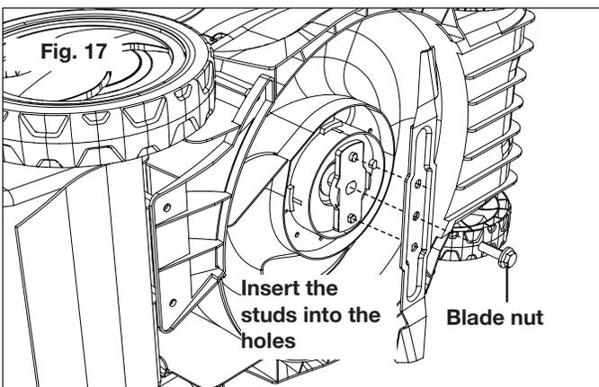
5. Fit the new blade on the same position by inserting the 2 small studs on the motor inside the holes of the blade, and secure with the original blade nut.
