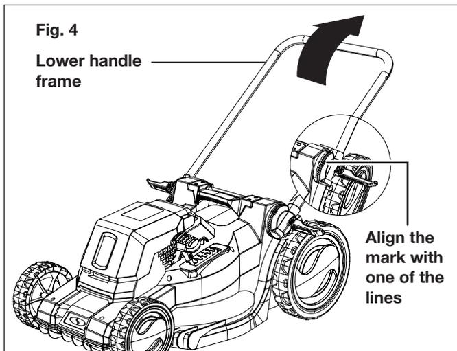
**NOTE:** The lawn mower is equipped with 3 handle heights, as shown below (Fig. 5).
