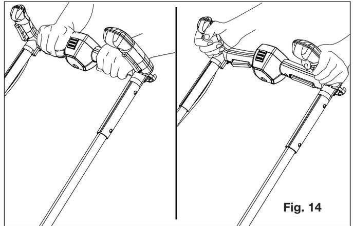
3. To stop the mower, release the On/Off switch buttons.
