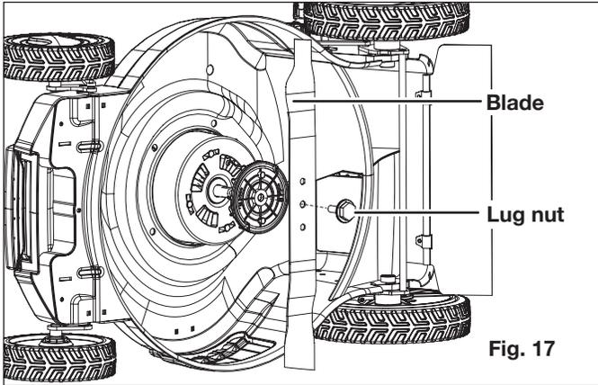
5. Fit the new blade on the same position and secure with the original lug nut (Fig. 18).
