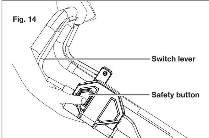
3. Once the machine powers on, release the safety lock button and proceed with operation.
