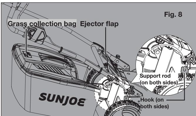
3. Release the ejector flap so that it rests on the grass bag. (Fig. 9).
