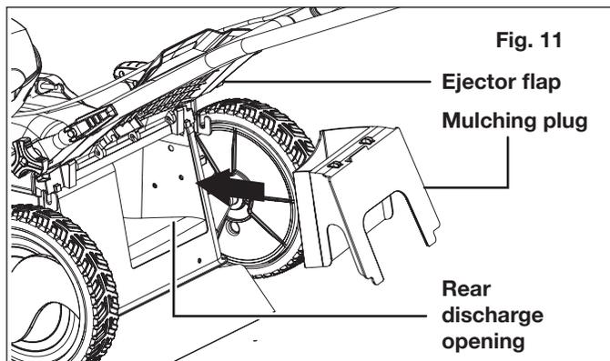
3. Release the ejector flap.
