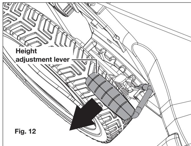
3. Insert the lever into the desired slot.
