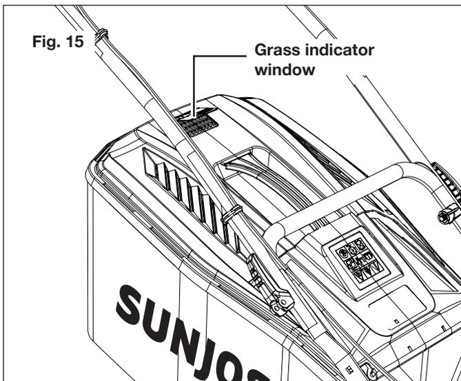
**NOTE:** To ensure that the filling level indicator functions properly, keep the holes under the flap clean and permeable.
