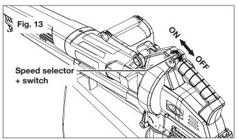
**3.** To stop the tool, slide the speed selector + switch backward until the notches in the housing align with the 0 position (Fig. 14).
