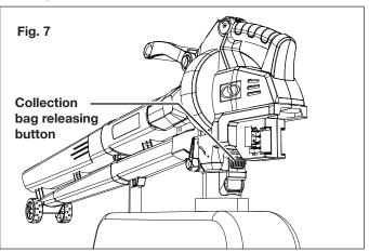
**WARNING!** DO NOT OPERATE THIS TOOL AS A VACUUM/MULCHER WITH COLLECTION BAG REMOVED. Serious injury from the fan or flying debris could result.
