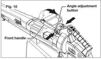
**2.** Release the angle adjustment buttons and the front handle will reset to lock into position automatically.
