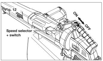
**3.** To stop the tool, slide the speed selector + switch backward until the notches in the housing align with the 0 position (Fig. 13).
