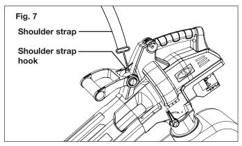
To adjust the length of the strap, push it from one end to form a loop above, and let out as needed, then pull the strap from the other side to tighten (Figs. 8 – 9).
