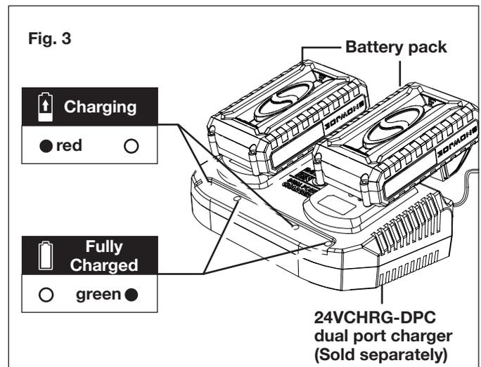
3. The battery indicator LEDs will illuminate one by one during the charging process. Unplug the charger immediately when the 3 LEDs are all illuminated.
