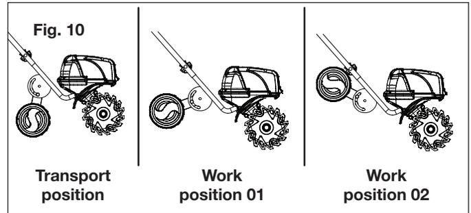
2. To adjust the wheel position, push the wheel adjustment knob while moving it to the slot for desired position; let go of the knob and make sure it locks into position (Fig. 11).
