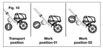
2. To adjust the wheel position, push the wheel adjustment knob while moving it to the slot for desired position; let go of the knob and make sure it locks into position (Fig. 11).
