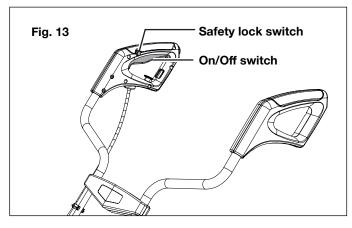
3. To switch OFF, release the ON/OFF switch (Fig. 13).
