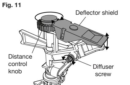
**NOTE:** The spray distance will depend heavily on your water pressure. Do not exceed this product's maximum rated pressure of 100 PSI.
