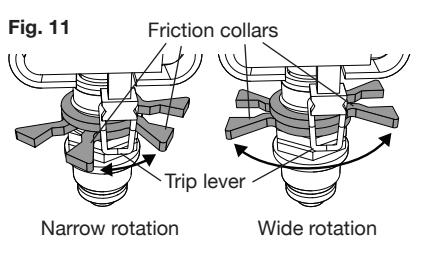
2. Flip the trip lever up out of the way of the friction collars to achieve full 360° rotation (Fig. 12).
