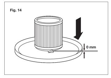
Fit the wire filter basket over the pleated filter and turn it clockwise until it stops. The wire filter basket tabs must cover and depress the safety stop switch.
