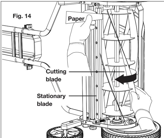
9. If most of the blades cut on both ends, the cutting system is set correctly. If all or most of the blades do not cut on one or both ends, the cutting system needs to be adjusted. Follow the instructions for adjusting the blade below.
