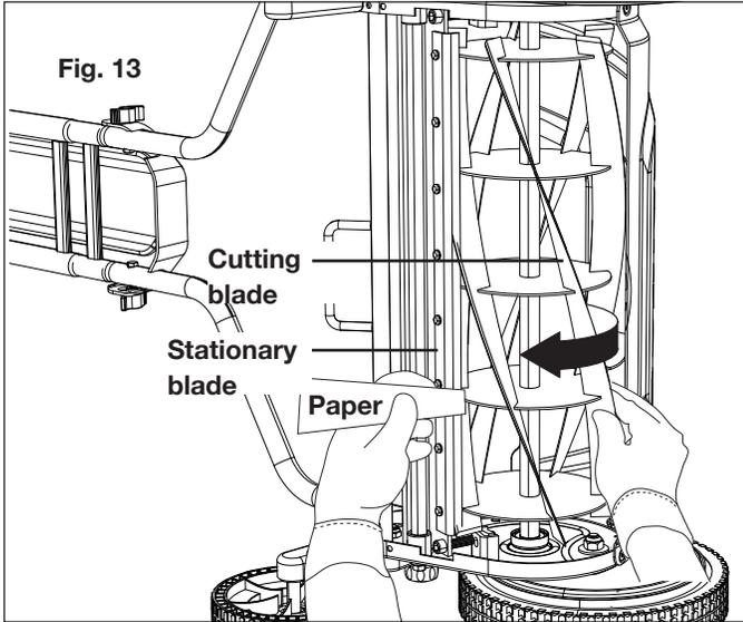
7. Continue to feed the paper into the reel horizontally half an inch at a time to check the other blades.
