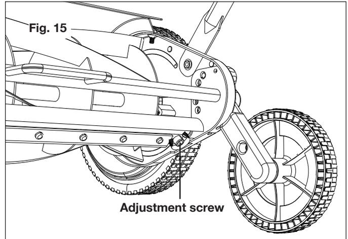
**⚠ WARNING!** Do not overtighten the adjustment screws as this could damage the cutting bar. Both screws must be tight on final adjustment.
