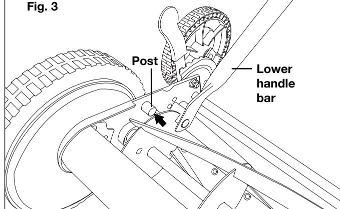
4. Pull both sides of the lower handle bars over the posts on the mower body. Press inward on the handle bars to ensure a secure fit over the posts.
