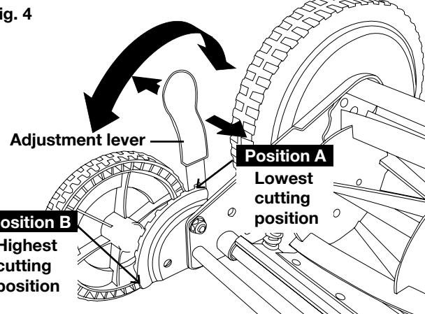
4. Other cutting heights are achieved by moving the adjustment levers to the settings between the highest and lowest positions.
