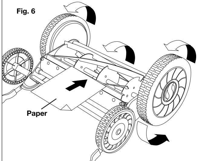
3. All the blades should slice the paper evenly along the entire length of the cutting bar while the reel is turned smoothly.
