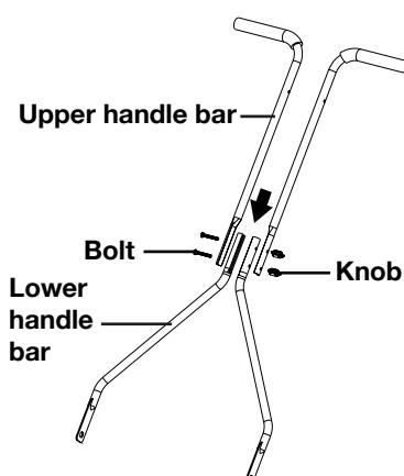
2. Attach the two upper handle bars to each other using one bolt and knob provided. Tighten the knob to ensure a secure fit (Fig. 2).
