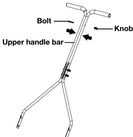
3. After assembling the handle, line up the holes at the lower end of each handle arm with the short posts that extend from the side plates of the mower base (Fig. 3).
