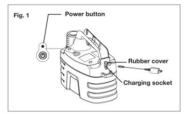
The light on the power button will shine red when it is charging and green once it is complete. The charger turns off automatically once the battery is fully charged. The green light will turn off after 5 hours (Fig. 1). **CAUTION!** FIRE HAZARD. When disconnecting the charger from the battery, be sure to unplug the charger from the outlet first, then disconnect the charger from the battery
