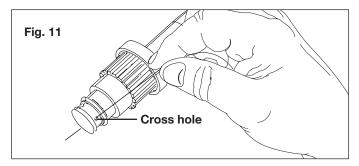
Wipe the nozzle and cross holes with a clean dry cloth and reinstall the nozzle.
