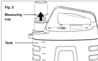
**3.** Fill the tank with the desired amount of water (up to 2 gallons).
