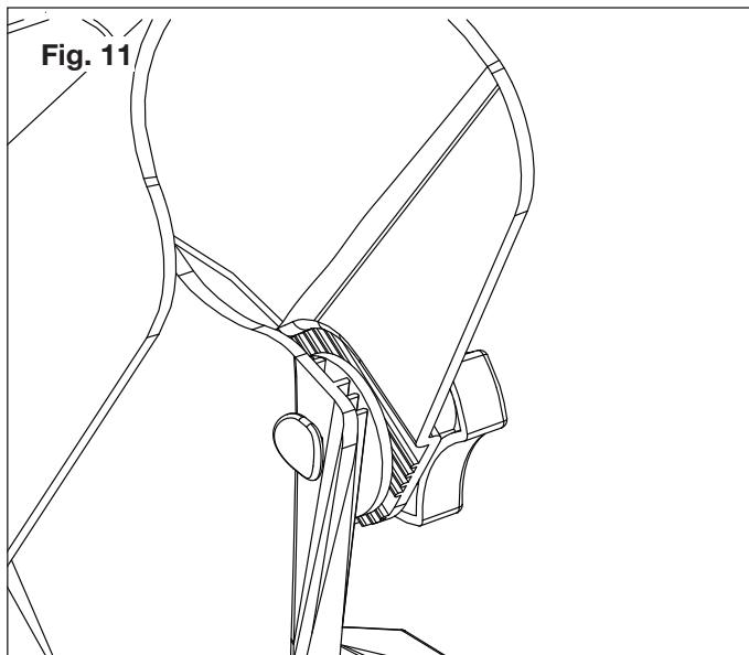
3. Turn the crank knob clockwise to ensure the discharge chute and deflector are in position.
