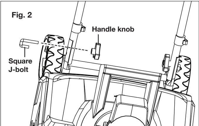
3. Secure the middle handle assembly to the lower handle using 2 knobs and 2 J-bolts. Install the knobs on the inside of the unit, and tighten (Fig. 3).
