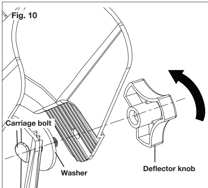
2. Secure the carriage bolts and knobs. Make sure the knobs are tightened (Fig. 11).
