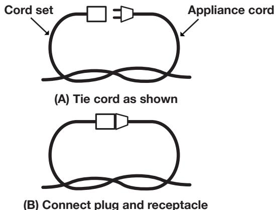
5. Do not abuse the cord. Never pull the snow thrower by the cord or yank the cord to disconnect it from the receptacle. Keep the cord away from heat, oil, and sharp edges.
