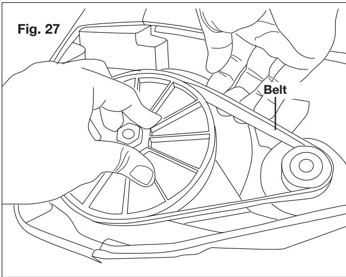
3. Put the belt on the drive pulley first and then place the belt at the lower end of the auger pulley (Fig. 28).
