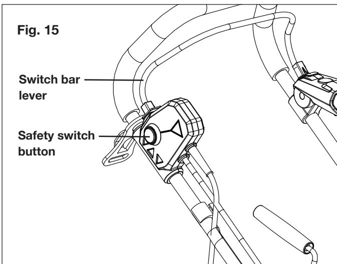
2. Once the snow thrower starts, release the safety switch button and proceed with operation.
