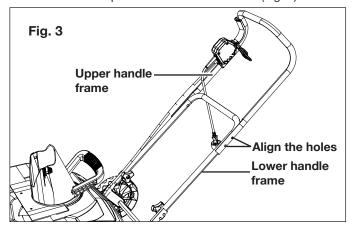
**4.** Secure the upper handle frame to the lower handle frame with 2 sets of knob and carriage bolt like shown (Fig. 4). Make sure the knobs are tightened.
