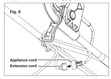
4. Note that the snow thrower has a polarized male plug – one prong in the plug is slightly longer and wider than the other (Fig. 10). The extension cord female end should be likewise polarized so that the extension cord fits snugly into the appliance plug.
