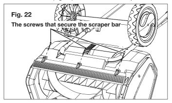
3. Install the new scraper bar and fasten it securely to the snow thrower with the 3 screws.
