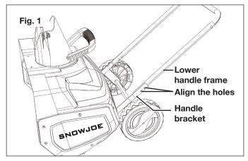
Secure the lower handle frame to the handle brackets with the 2 sets of knob and J-bolt, like shown (Fig. 2). Make sure the knobs are tightened.
