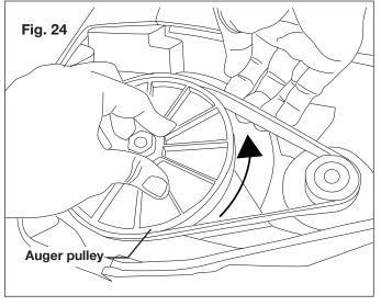
**3.** Put the belt on the drive pulley first and then place the belt at the lower end of the auger pulley (Fig. 25).
