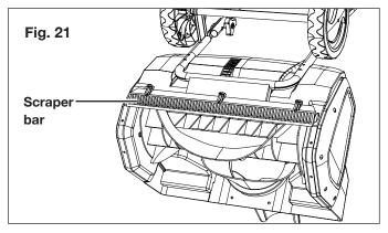
2. Remove the 3 screws that secure the scraper bar to the snow thrower (Fig. 22). Remove the old scraper bar.
