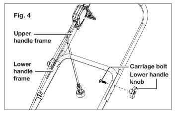
5. Clip the cable in the cable clips on the lower handle to secure the cable.
