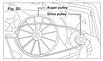
4. Use your right hand to press the belt with ribbed side down. While holding the belt down with your right hand, use your left hand to turn the auger forward so that the auger pulley rotates in a clockwise direction. The belt will be gradually pushed down onto the pulley. When the belt is seated on the pulley, adjust it so that the ribs of the belt match the grooves on the pulley (Fig. 26).
