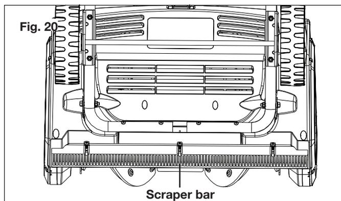
2. Detach the worn scraper bar from the snow thrower by removing the 3 screws that hold it in place (Fig. 21).
