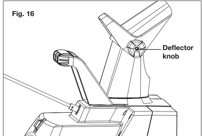
2. The chute deflector on the top of the discharge chute controls the height of the snow stream. Loosen the knob to raise or lower the deflector to the desired height of snow you wish to throw. Tighten the knob to secure the deflector (Fig. 16).
