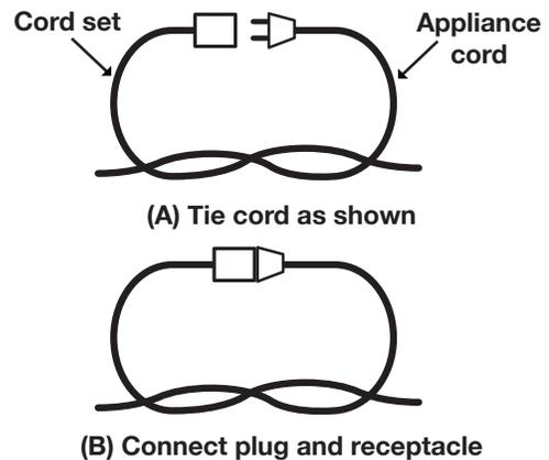
5. Do not abuse the cord. Never pull the snow thrower by the cord or yank the cord to disconnect it from the receptacle. Keep the cord away from heat, oil, and sharp edges.
