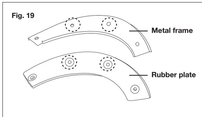
3. Attach the new rubber plate onto the metal frame by replacing and tightening the middle four sets of nuts and bolts (Fig. 19).
