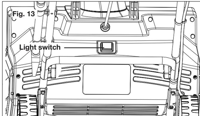
**NOTE:** The lights will only turn ON when the snow thrower is running. After finishing your work session, REMEMBER to TURN OFF the light switch.
