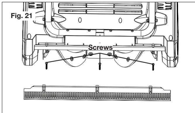
3. Install the new scraper bar and fasten it securely to the snow thrower with the 3 screws (Fig. 21).
