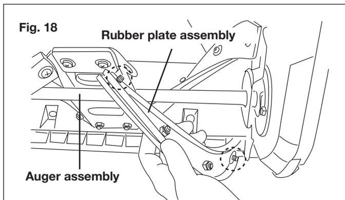
2. Loosen the middle two sets of nuts and bolts to detach the worn rubber plate from the metal frame (Fig. 19).
