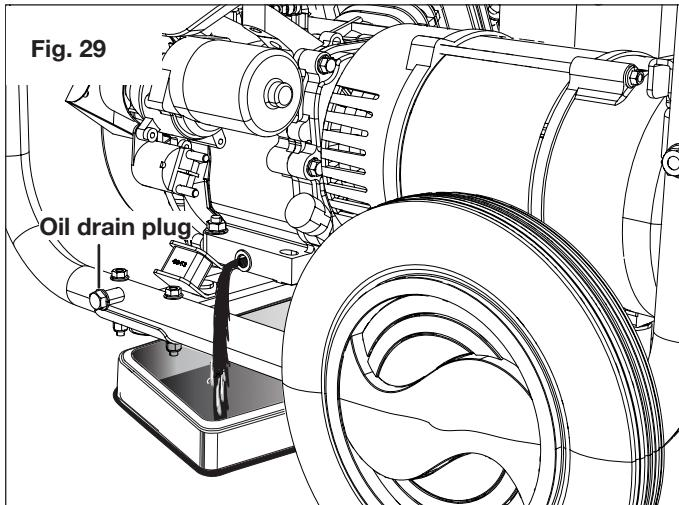
**⚠️WARNING!** Drain the lubricant while the engine is still warm but not hot. Warm lubricant will drain quickly and more completely.
