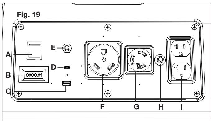
**A. Engine switch** – Use the engine switch to start the generator.
