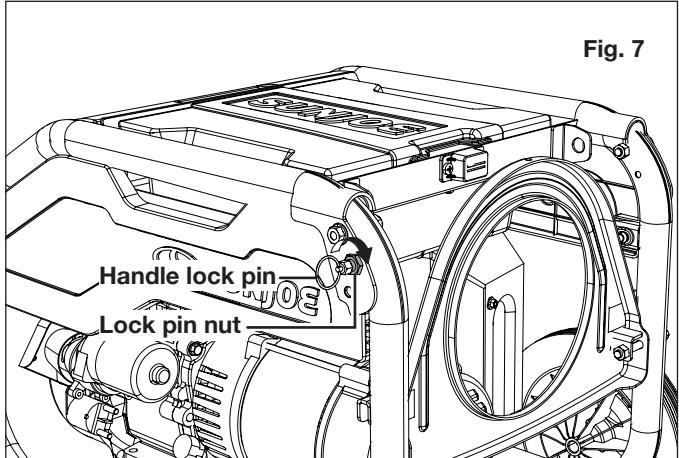
3. To extend the handle, pull the lock pin ring to unlock the handle, and turn the handle up to the transporting position. Release the ring to lock the handle in place. To
