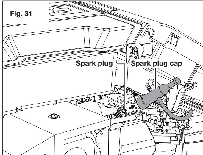
3. Clean any dirt from around base of spark plug.
