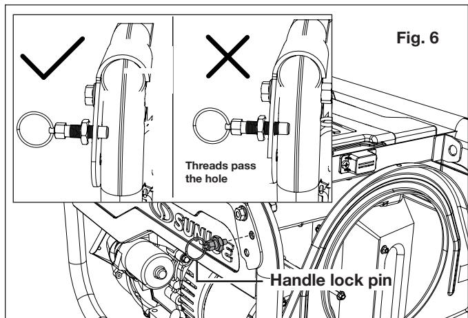
2. Holding the lock pin in place, use a wrench to turn the nut on the lock pin clockwise to secure (Fig. 7).
