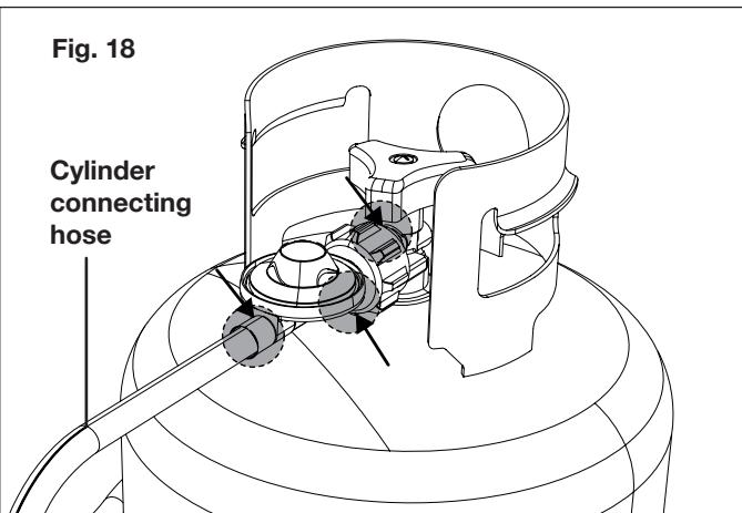
3. Turn on the cylinder. Inspect the connections and look for bubbles. If no bubbles appear, the connection is safe. If bubbles appear, there is leakage. Loosen and re-tighten this connection. If there is still a leak, turn off the cylinder and contact the Snow Joe® + Sun Joe® customer service center at 1-866-SNOWJOE (1-866-766-9563).
