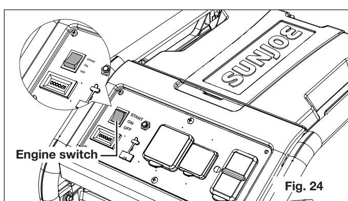
**NOTE:** The battery may require charging before the generator can be electric started. In this case, start the engine by recoil start described below.
