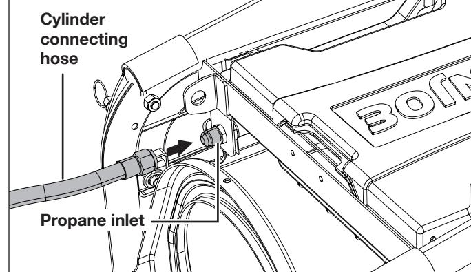
2. Lower the cylinder bracket completely. Place a propane cylinder (not included) into the bracket, making sure the bottom of the cylinder is placed securely in the opening in the bracket. To secure the cylinder, place the cylinder strap around the cylinder and connect to the hook on the generator frame as shown (Fig. 15).
