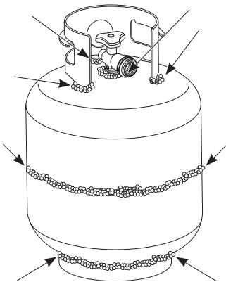
4. If bubbles show up, there is a leak. Do not use or move the propane cylinder. Contact a gas supplier or the fire department!
