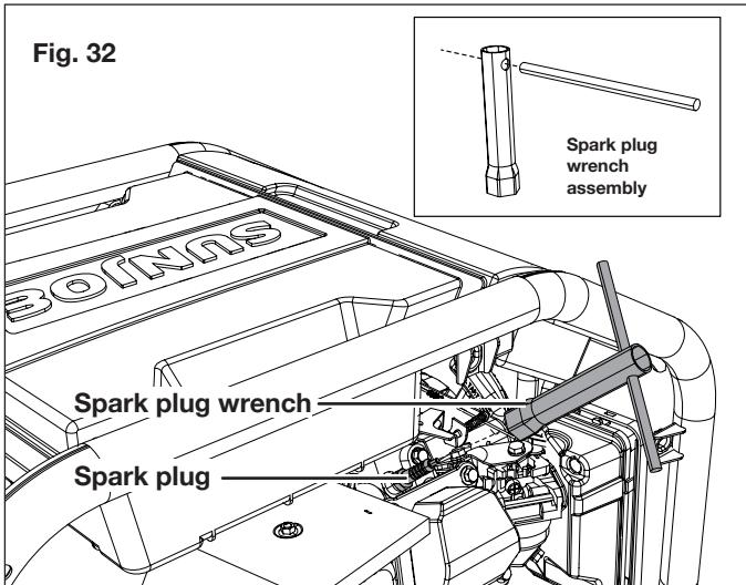
5. Inspect spark plug for damage, and clean with a wire brush before reinstalling. If insulator is cracked or chipped, spark plug should be replaced.
