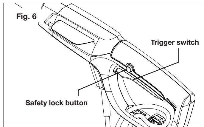
2. To turn the tool OFF, release the trigger switch (Fig. 6).
