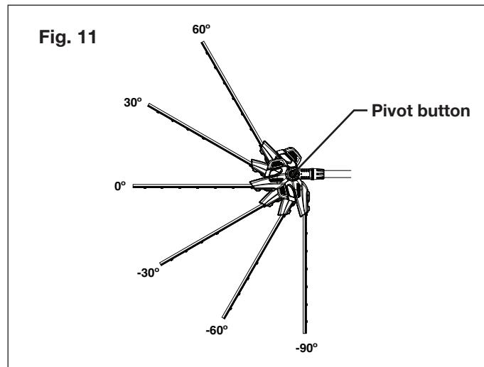
4. Ensure the trimmer head is locked in position when the button is released.
