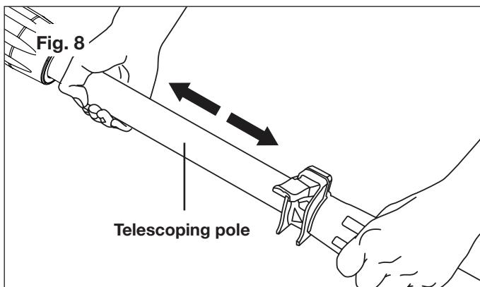
4. Lock the pole in position by closing the cam-lock (Fig. 9), and ensure that the pole is secure. If the pole telescopes when the cam-lock is closed, the nut may need tightening.
