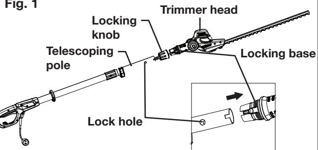
3. Slide the locking knob onto the locking base and rotate the locking knob clockwise to secure (Fig. 2).
