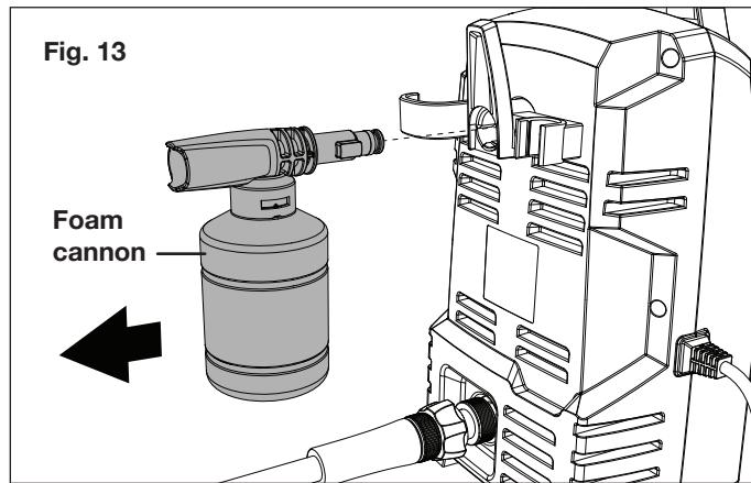
2. Twist counter-clockwise to remove the spray nozzle. Fill the foam cannon bottle or mix as recommended according to the detergent instructions, before replacing the spray nozzle back onto the bottle (Fig. 14).
