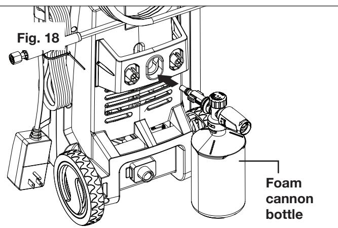
2. Remove the cap. Fill the bottle or mix as recommended by detergent instructions (Fig. 19), and secure the cap back into place. Replace it back on the unit.
