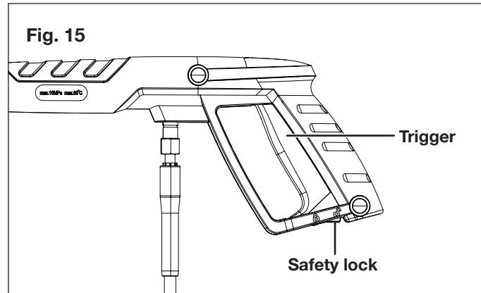
5. Keeping the trigger pressed, turn the switch to the ON (I) position to start the pressure washer.
