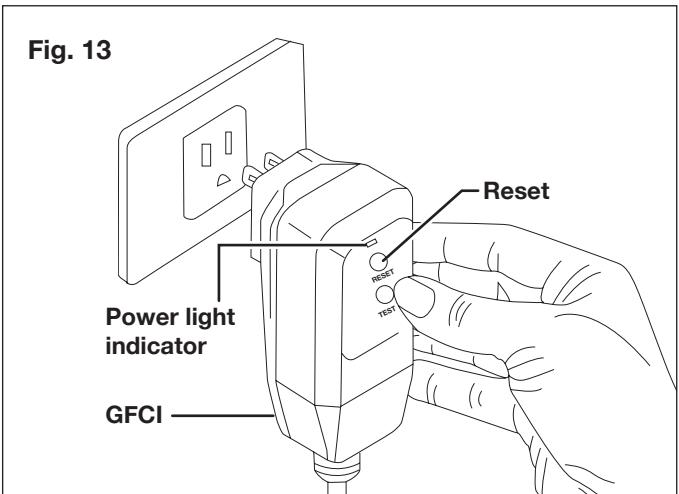
**NOTE:** The GFCI may need to be reset when first plugged into the electric outlet. Press the "Reset" button until the power light indicator on the GFCI illuminates.
