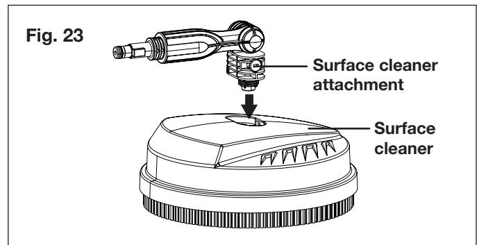
2. Flip the surface cleaner over and align the dual-nozzle rotating sprayer with the attachment of the surface cleaner (Fig. 24).
