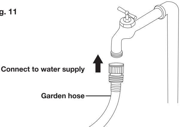
**⚠️WARNING!** The intake water temperature must not exceed 104°F/40°C. The water supply must not exceed 0.7 MPa.
