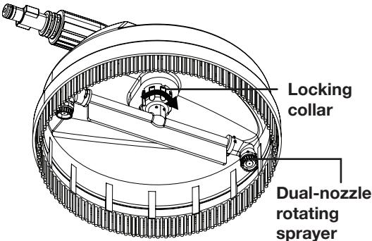
4. Fit the surface cleaner extention wand into the surface cleaner attachment and turn the rotatable end-piece of the wand until the two parts are completely locked together (Fig. 26).
