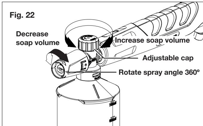
**WARNING!** Do not adjust the foam cannon while the trigger is squeezed. Failure to do so could result in damage.
