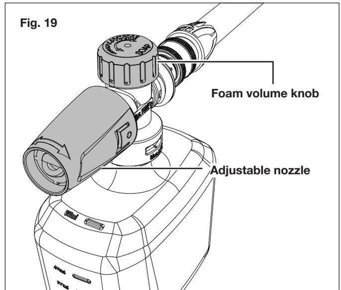
**⚠️ WARNING!** Do not adjust the foam cannon while the trigger is engaged. Doing so may result in damage.
