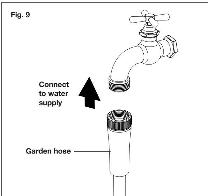
**⚠ WARNING!** Do not connect to potable water system.
