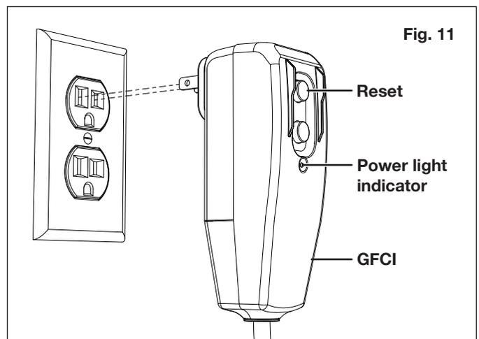
**NOTE:** The GFCI may need to be reset when first plugged into the electric outlet. Press the “Reset” button until the power light indicator on the GFCI illuminates when plugged in.
