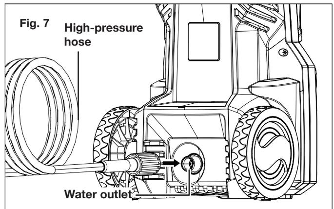
**⚠ WARNING!** Keep hose away from sharp objects. Bursting hoses may cause injury. Examine hoses regularly and replace if damaged. Do not attempt to mend a damaged hose.
