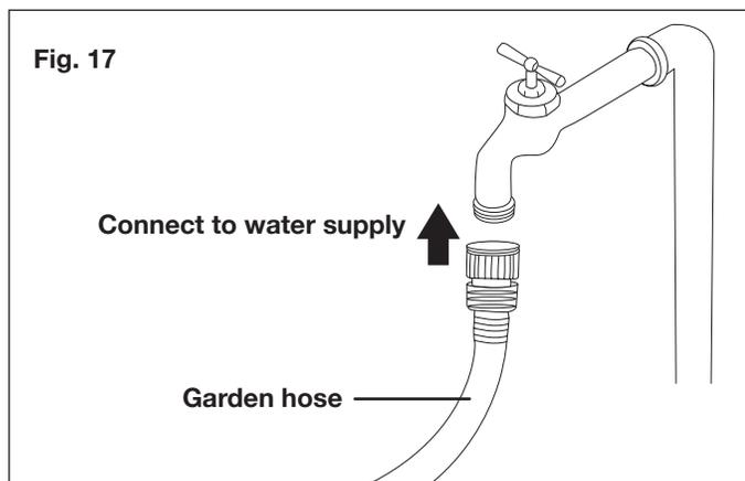
**⚠️ WARNING!** The intake water temperature must not exceed 104°F/40°C. The water supply must not exceed 0.7 MPa.
