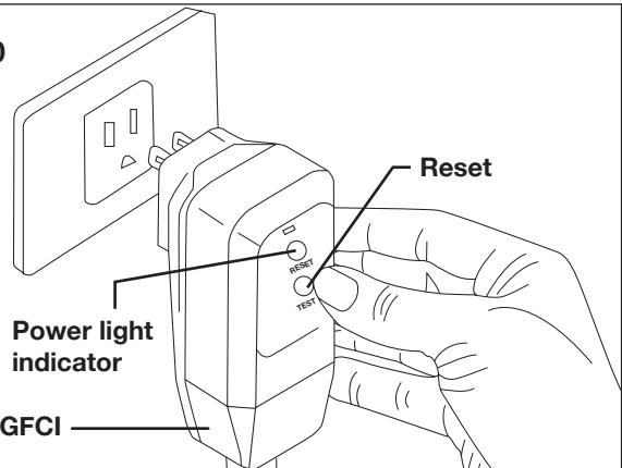
**NOTE:** The GFCI may need to be reset when first plugged into the electric outlet. Press the "Reset" button until the power light indicator on the GFCI illuminates when plugged in.
