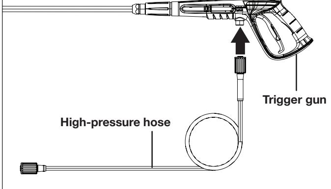
5. Connect the other end of high-pressure hose to the water outlet on the washer (Fig. 5).
