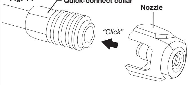
To disconnect a nozzle from the spray wand once the cleaning job is complete:
