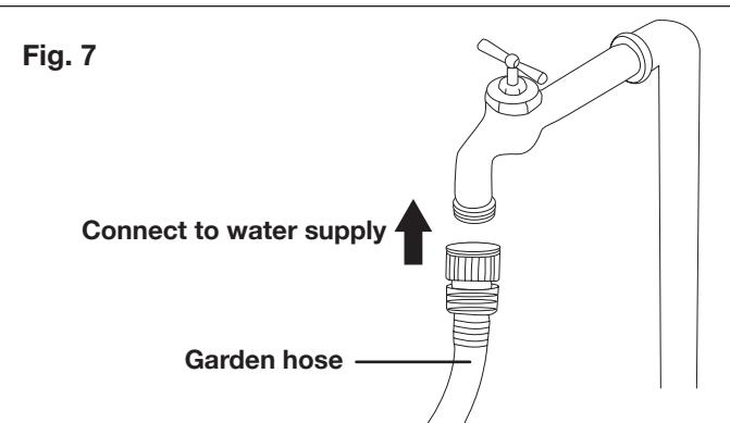
**⚠️ WARNING!** Keep hose away from sharp objects. Bursting hoses may cause injury. Examine hoses regularly and replace if damaged. Do not attempt to mend a damaged hose.
