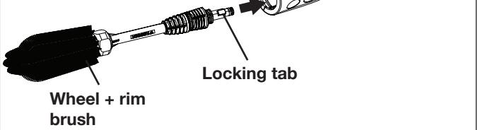
3. Once aligned, push the Wheel + rim brush into the trigger gun, twist counterclockwise to lock into place.
