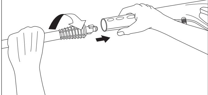
8. Connect the high-pressure hose to the trigger gun (Fig. 8).
