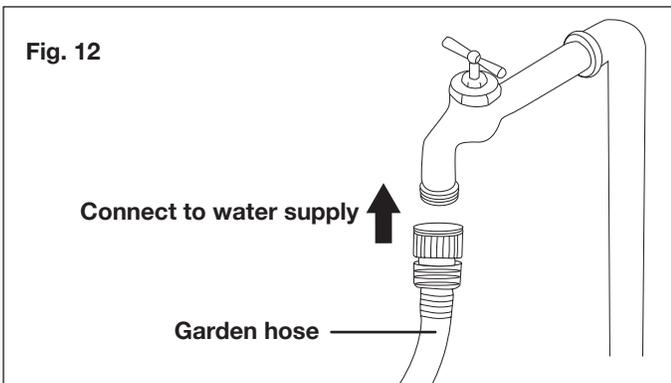
**⚠ WARNING!** Do not connect to potable water system.
