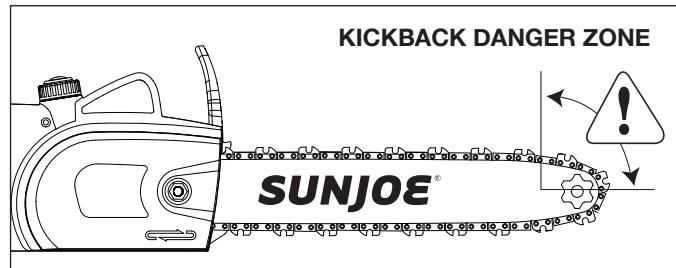
Kickback may occur when the nose or tip of the guide bar touches an object, or when the wood closes in and pinches the saw chain in the cut. Tip contact in some cases may cause a sudden reverse reaction, kicking the guide bar up and back towards the operator.
