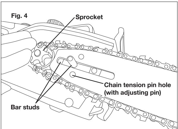
**NOTE:** If the adjusting pin will not reach the chain tension pin hole, turn the chain tensioning screw counter-clockwise until the pin hole aligns with the adjusting pin (Fig. 5).
