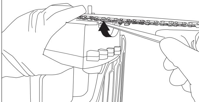
2. The tension is correct when the drive links on the chain do not slip out of the chain guide on the bar when the chain is pulled up from the middle of the bar (Fig. 10).
