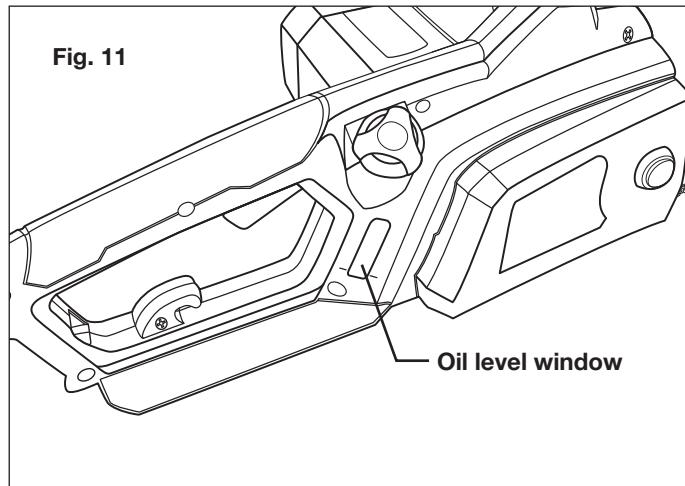
**NOTE:** Your electric chain saw is equipped with an automatic oil pump for bar and chain oiling. You must add bar and chain oil or your chain saw will malfunction.
