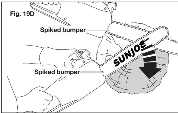
After completing the cut, wait for the saw chain to stop before you move the chain saw. Always stop the motor before moving from tree to tree.
