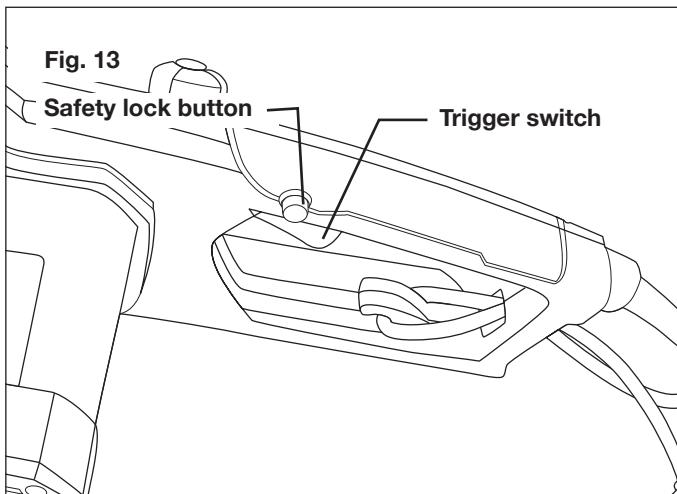
6. To turn the tool OFF, release the trigger switch (Fig. 13).
