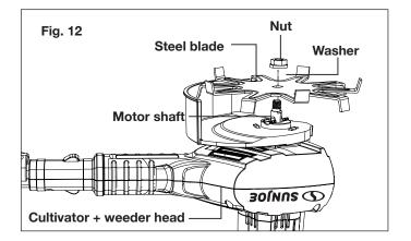
**3.** Insert the new steel blade on the motor shaft. Make sure to align the notches on the blade hole with the notches on the motor shaft, and press the blade firmly on the motor shaft until it sits flush (Fig. 13).
