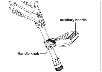
**2.** Adjust the auxiliary handle to a comfortable working position (Fig. 8).
