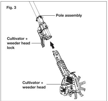
Flip up the cultivator + weeder head lock to lock the cultivator + weeder head in place (Fig. 4).
