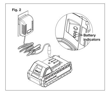
**3.** The battery will take approximately 1 hour and 20 minutes to charge. The battery indicator LEDs will twinkle and illuminate one by one during the charging process. Unplug the charger immediately when the 3 LEDs are all illuminated.
