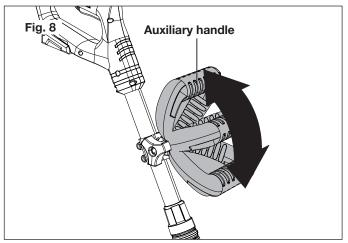
**3.** Turn the handle knob back to lock the auxiliary handle in position.
