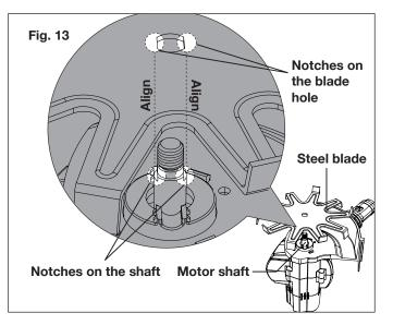
**Note:** Failure to align the notches will cause the blade to be unstable and wobble during use.
