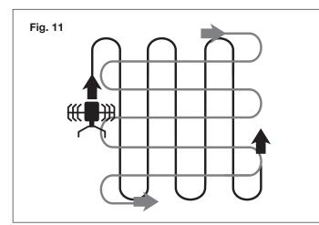
• Pay special attention when changing direction. Apply light pressure to the handle in order to lift the blade and facilitate the turn. Turn the product around using the wheels as a guide. Gradually release pressure on the handle and move the blade back to the ground.
