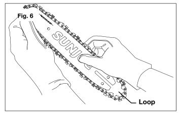
6. Hold the chain in position on the bar and place the loop around the sprocket. Fit the bar against the mounting surface so that the bar stud is in the long slot of the bar and the adjusting pin is in the chain tension pin hole (Fig. 7).
