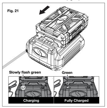
**NOTE:** If the green light is off while the red light flashes slowly, this indicates a temperature abnormality (i.e. that the battery pack is too hot). If the green light is off while the red light flashes rapidly, this indicates there's something wrong with the charger or the battery. Wait for a while and try to reinsert the battery into the charger. If the situation still persists, contact Snow Joe® + Sun Joe® customer service at 1-866-SNOWJOE (1-866-766-9563).
