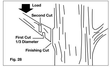
Now make your finishing cut from the topside of the branch smoothly and neatly against the main member so the bark will grow back to seal the wound.  Release the ON/OFF switch as soon as the cut is completed. Failure to follow proper cutting procedures will result in the bar and chain binding and becoming pinched or trapped in the limb.
