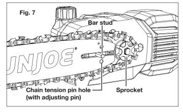
**NOTE:** To align the adjusting pin with the pin hole, move the adjusting pin backward as needed by adjusting the chain tensioner screw counterclockwise with the supplied blade screwdriver (Fig. 8).
