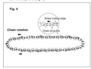
5. Starting at the tip, mount the chain drive links into the bar groove, leaving a loop at the back of the bar. The chain will loosely fit until it is placed on the sprocket. (Figs. 5 & 6)
