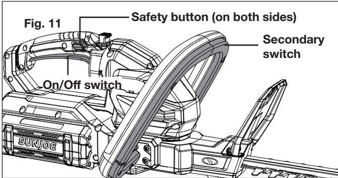
3. To turn the tool OFF, move the hedge trimmer away from cutting area, and release one of the switches (Fig. 11).
