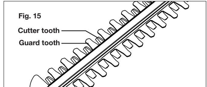
2. Stop the motor and remove the battery. Clamp the blade in a vise.
