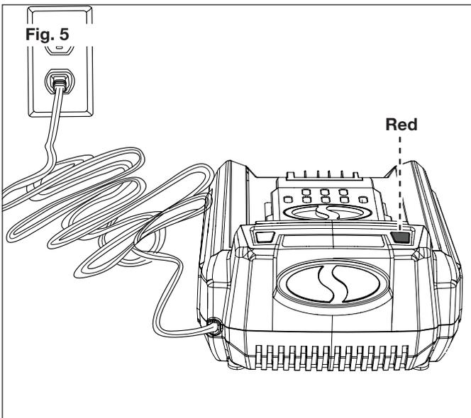
**⚠ CAUTION!** Charger iON100V-RCH is rated for 100 – 120 volt AC only. DO NOT plug the charger into any outlet that will provide power with a higher voltage. Over voltage charging will be harmful to both the battery and charger, and may cause the charger to burn out.
