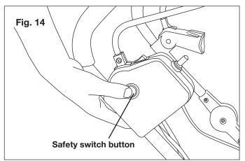
**4.** While depressing the safety switch button, pull the ON/OFF switch bar lever toward you. Once the machine powers on, release the safety switch button and proceed with operation (Fig. 15).
