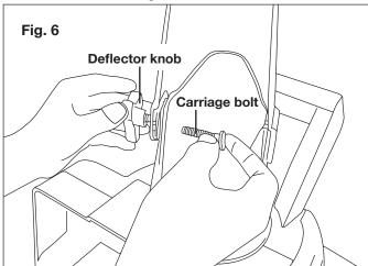
NOTE: Do not overtighten the knobs.
