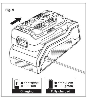
**NOTE:** If the top light remains green while the bottom light alternately flashes red and green, this indicates a temperature abnormality (i.e. that the battery pack is either too hot or too cold). If there is only a red blinking light, this indicates that something is wrong with the battery. Contact the Snow Joe<sup>®</sup> + Sun Joe<sup>®</sup> customer service center at 1-866-SNOW-JOE (1-866-766-9563) for assistance.
