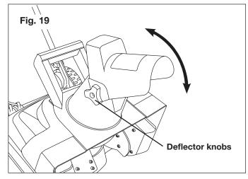
**WARNING!** Make sure that the chute deflector locks completely onto the discharge chute. An opening between the discharge chute and the chute deflector may allow foreign objects picked up by the snow blower to be thrown in the direction of the operator, which can cause serious bodily injury.
