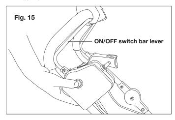
To power off, release your grip on the ON/OFF switch bar lever.
