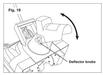
**WARNING!** Make sure that the chute deflector locks completely onto the discharge chute. An opening between the discharge chute and the chute deflector may allow foreign objects picked up by the snow blower to be thrown in the direction of the operator, which can cause serious bodily injury.
