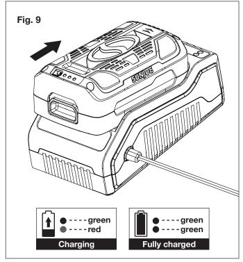
**NOTE:** If the top light remains green while the bottom light alternately flashes red and green, this indicates a temperature abnormality (i.e. that the battery pack is either too hot or too cold). If there is only a red blinking light, this indicates that something is wrong with the battery. Contact the Snow Joe® + Sun Joe® customer service center at 1-866-SNOW-JOE (1-866-766-9563) for assistance.
