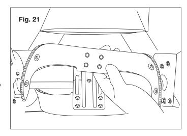
2. Install the new rubber plate assembly by tightening the 8 sets of nuts and bolts on both sides (Fig. 20).
