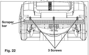
2. Detach the worn scraper bar from the snow blower by removing the 3 screws that hold it in place (Fig. 23).
