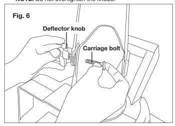
Raise or lower the chute deflector by loosening and tightening the deflector knobs to achieve the desired snow stream height.
