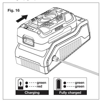
**NOTE:** If the top light remains green while the bottom light alternately flashes red and green, this indicates a temperature abnormality (i.e. that the battery pack is either too hot or too cold). If there is only a red blinking light, this indicates that something is wrong with the battery. Contact Snow Joe® + Sun Joe® customer service at 1-866-SNOWJOE (1-866-766-9563).
