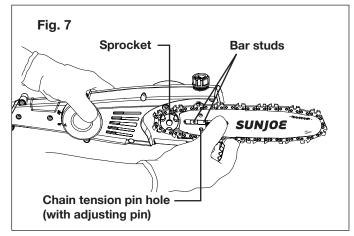
8. Adjust the chain tension as needed by adjusting the chain tensioner screw with the supplied flat-tip blade screwdriver. Make sure to align the chain tensioner screw with the pin hole (Fig. 8).
