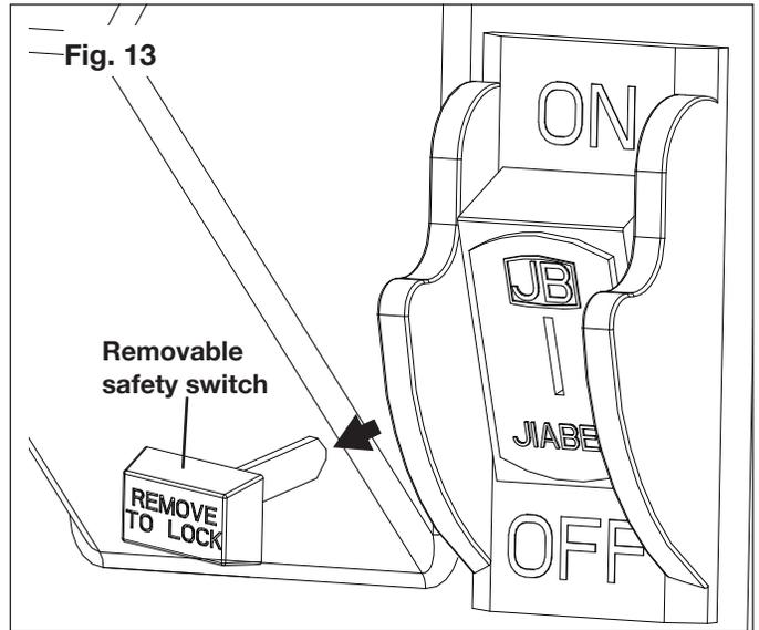
**NOTE:** As a safety precaution, the removable safety switch can be removed when you are not using the wood chipper + shredder to prevent children from starting it accidentally. The unit cannot be started when the safety switch is removed. Make sure to replace the removable safety switch before operation.
